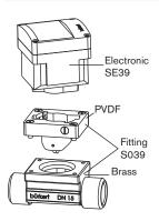
The flow controller 8039 is built up with an electronic module SE39 associated to a fitting S039 with integrated measurement paddle-wheel.
